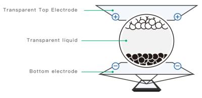
E-ink consists of millions of tiny microcapsules that are about the diameter of a human hair
