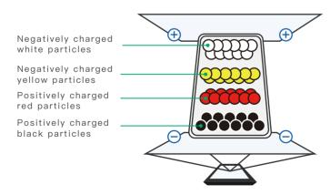
The ZKONG 4-particle system adds charged color particles in addition to white, enabling a broader color spectrum with black, white, red, and vellow
